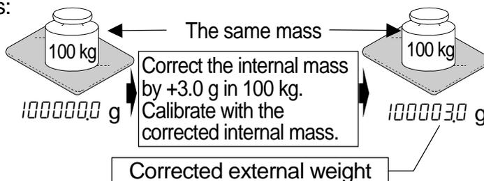
Step 1 Calibrate the balance using the internal mass. (one-touch calibration).
