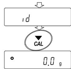
Step 10 Press the  key to return the weighing mode.
