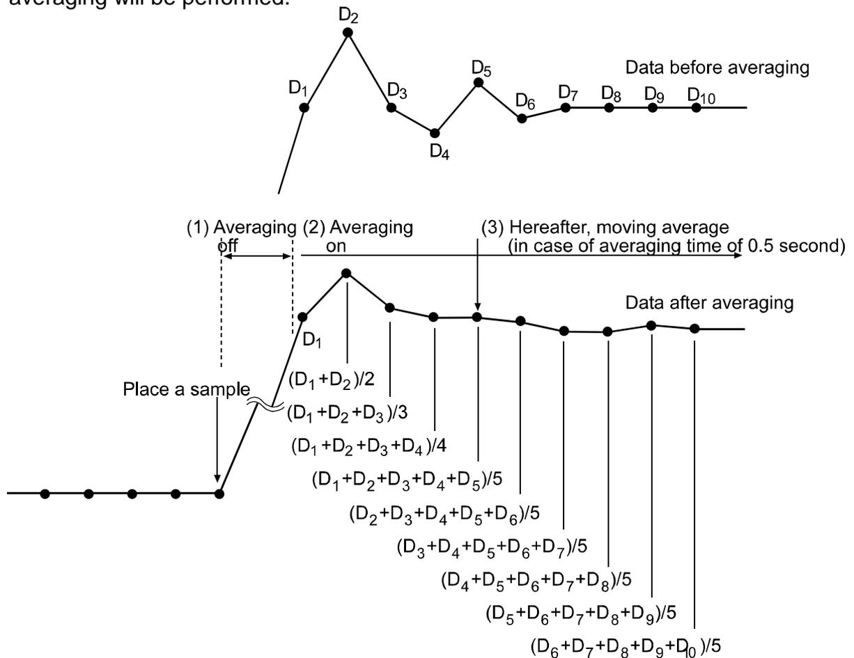
When a small amount of sample is weighed or is filled, the fluctuation of a weight value is too small to be beyond the selected range and the averaging operation is not disabled. Consequently moving averaging is always performed and it takes a longer time to reach the final weight value. Under such a situation, change the setting of " $F l-b$ " to a smaller range. But please note that the smaller the range is, the more prone to external disturbance the value will become.
