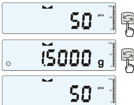
When special function e.g. *PCS* is turned on, using ↻ key enables to go back to standard weighing mode.
