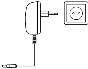
Plug feeder into 230V power supply socket. When the pan is empty plug feeder output connector into 12V socket at back of the balance. Autotests and internal calibration will be performed.
