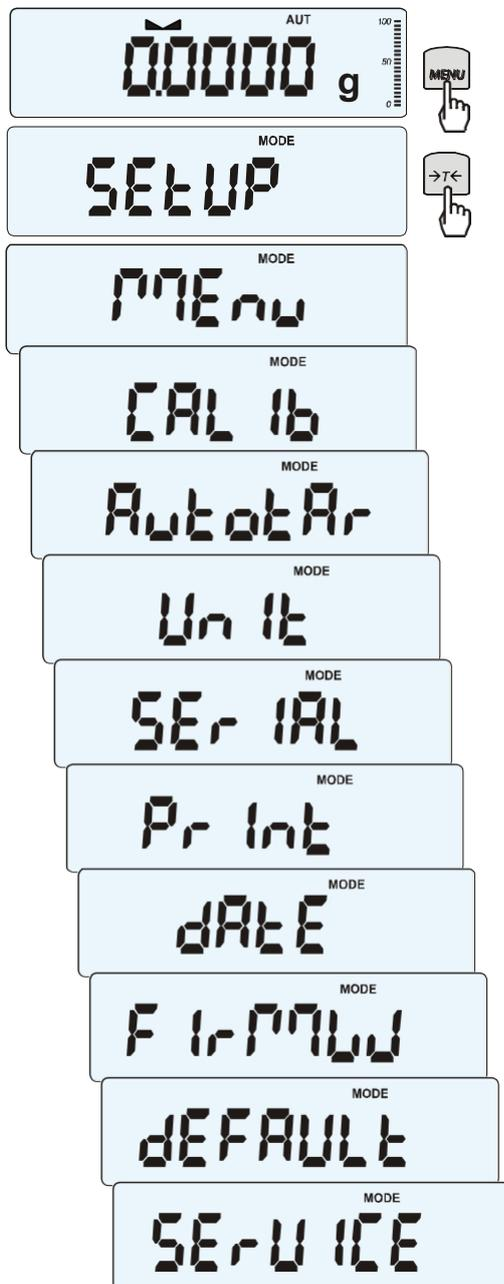
*SEtUP* contains all options used for setting scale work mode:
