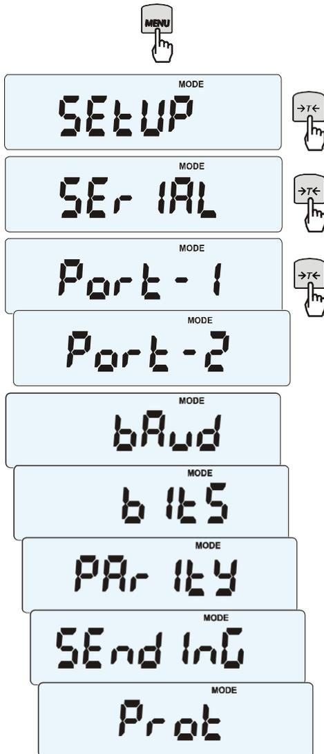
The function allows setting independently communication parameters of both of serial ports *Port-1* and *Port-2* (executed in RS232C, RS485, USB or LAN standard):
