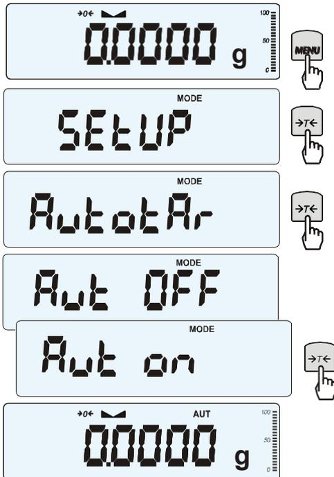
When the function is activated, the scale automatically ensures stable zero indication if the pan is empty or if zero indication was acquired by pressing **→T←** key.
