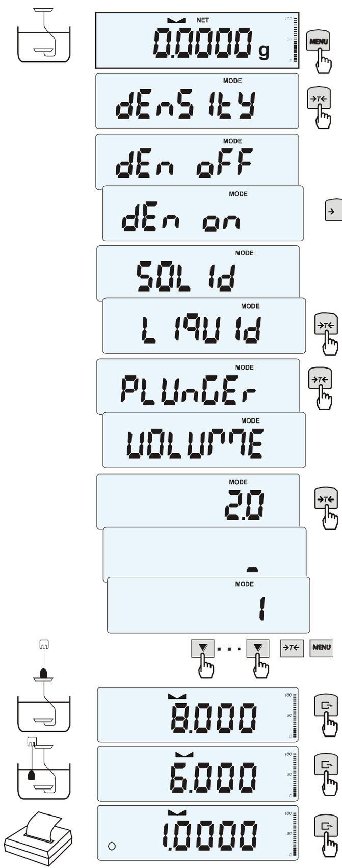
This function determines liquid density basing on plunger weight in air and in examined liquid with known volume, using the formula below:
