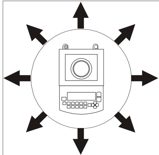
Location for the balance should be chosen with care in order to limit influence of the factors that can interrupt working balance. This location has to maintain proper temperature for working balance and necessary space for its operating. The balance should stay on stable table made of material that does not influence magnetically on the balance.
