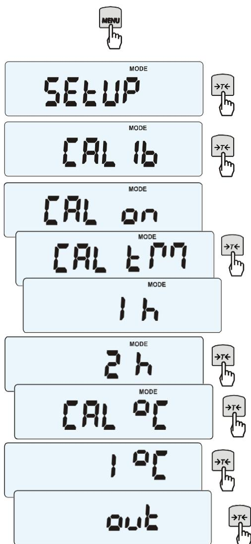
Press *MENU* key to display function menu and choose *CALib* function by pressing  $\rightarrow T \leftarrow$  key when it is displayed.
