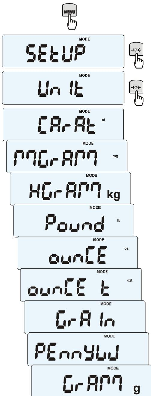
The function allows selecting weighing unit:
