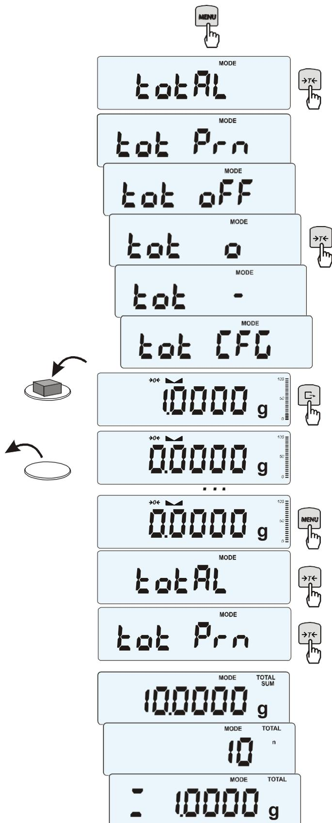
The function allows calculating total weight for series of measurements, which can be greater than scale capacity. It allows calculating total weight as well as average value.
