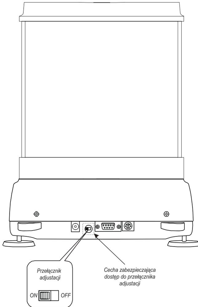
In balances comply with verification requirements performing calibration requires changing adjustment switch position, which is placed behind protecting mark (sticker) of a notified body. An access to the mark is possible only after removing the mark.
