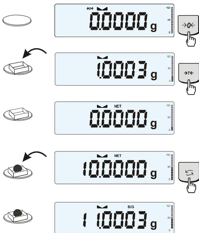
If the scale is not loaded and  $\rightarrow 0 \leftarrow$  indicator doesn't indicate, press  $\rightarrow 0 \leftarrow$  key.
