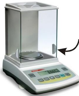
The function allows for separate weighing of several ingredients in one container with the possibility of reading current sum of all weighed ingredients.
