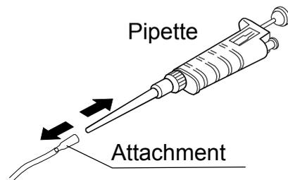
When measuring another pipette, press the **START** key again after connecting the pipette to be measured (return to “(2) Starting measurement”). The leak tester starts the measurement. At this time, the display is the measurement result.
