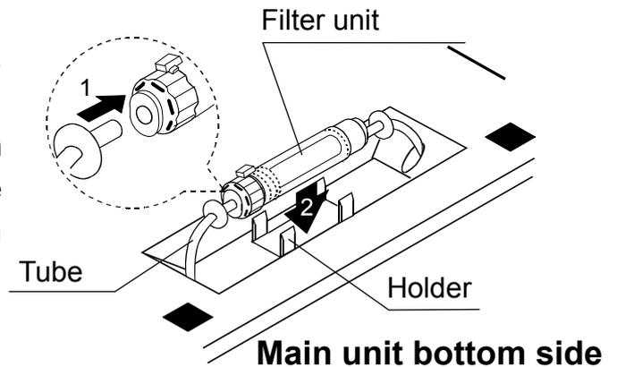
2. Install the filter unit into the holder.
