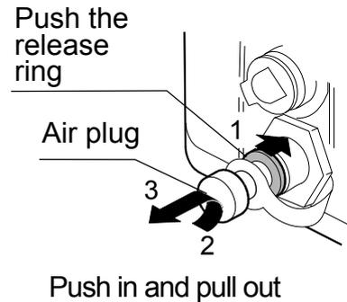
\* When connecting, confirm that the air plug or adapter tube is pushed in the connector hole firmly.
