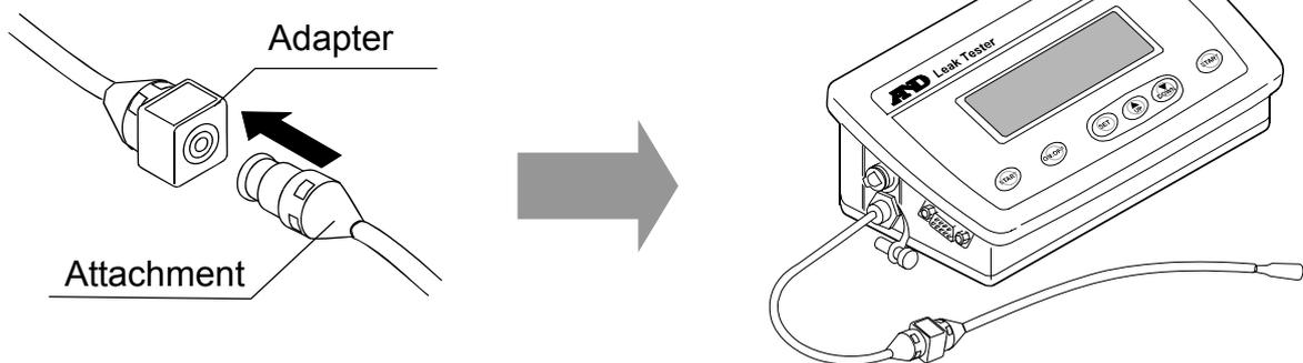
When the pipette does not match up with the attachment provided, replace the tip of the attachment with a tip that matches the pipette.
